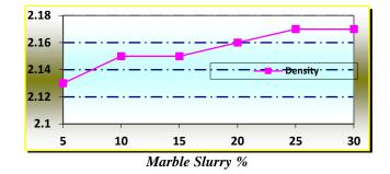
At water cement ratio 0.55 density of cement concrete for different % of marble slurry is more than water cement ratio 0.75 for similar % of marble slurry. But the mix at 0.55 w/c ratio is not workable while mix at 0.75 w/c ratio is workable showing good amount of density.
